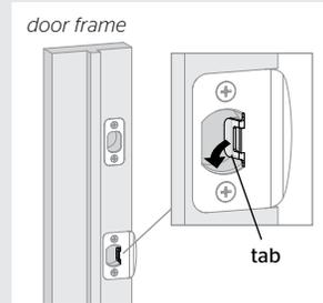
If your bottom strike does not have a tab, remove your bottom strike and replace it with the adjustable bottom strike in the kit.
