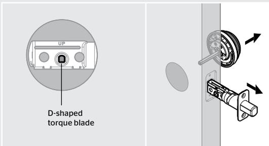
If your torque blade is another shape, the supplied latches will not work with your lock. Reinstall the interior parts on your door according to your lock's installation instructions, and stop here.
