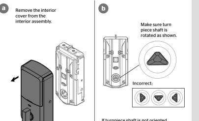
If turnpiece shaft is not oriented correctly, put the cover back on and
