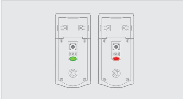
The Wireless Card LEDs are staying on.
