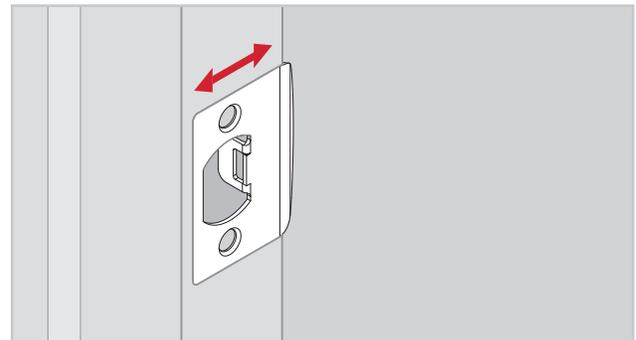
The hole in the door frame for the latch bolt is not drilled deep enough.
