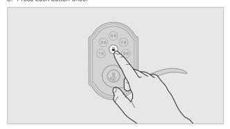
Press the Program button the number of times that corresponds to the user code position being programmed.
