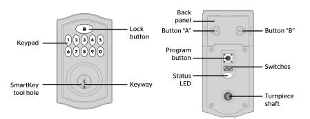
Note: When the cover is removed, the turnpiece shaft can be used to manually lock and unlock the door.
